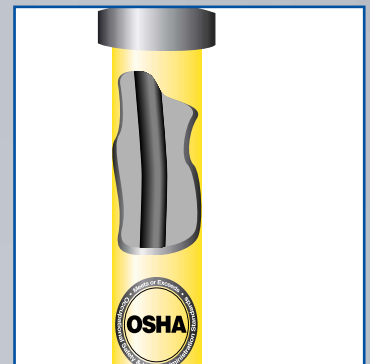
Power Cord Runs Inside The Pole
